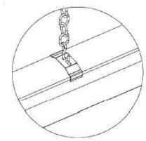
Suspension mounting is easy with mounting clips and chain included.
