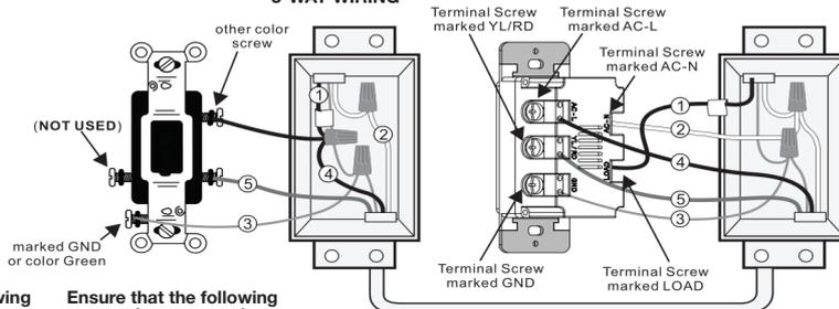
Note: A single pole or 3-way switch can be used alongside the smart switch.
